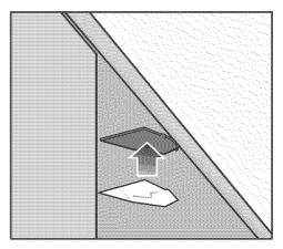
Press the optic indicator reflector into the reflector holder.
